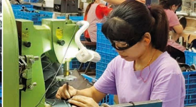
^ The worker punches holes for eyelets on the safety shoe.
